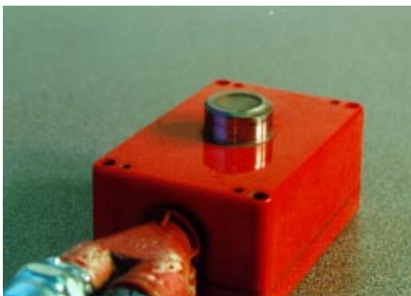
Here is an example of a spark detection FM 1/6 sensor obscured from abrasion. (Blinded.)
