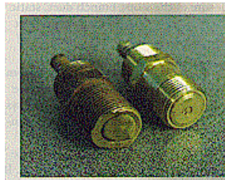
This photograph of spark detection extinguishment nozzles shows the excessive wear that comes from abrasion.
