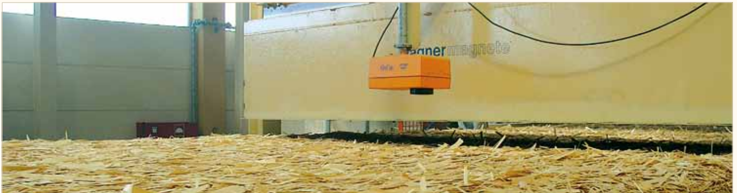
Moisture measurement after the forming line
