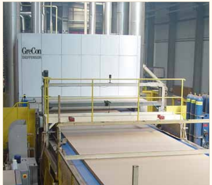
DIEFFENSOR in HDF line
