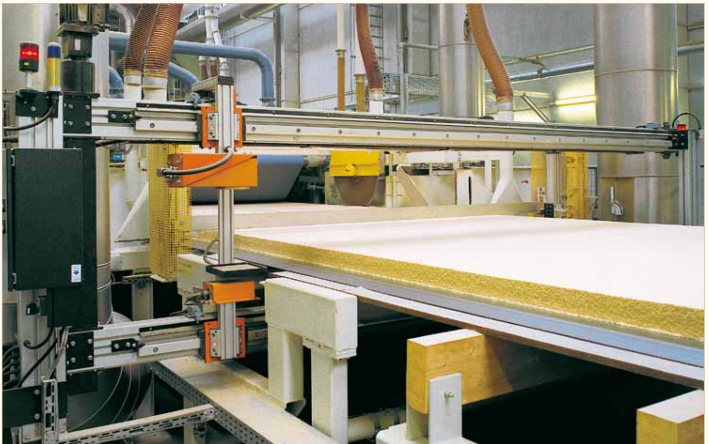
Measurement transducer in the calibration position
