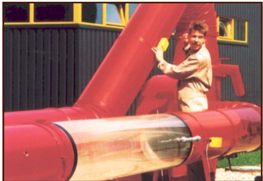
Testing a GreCon spark detection/extinguishment system
